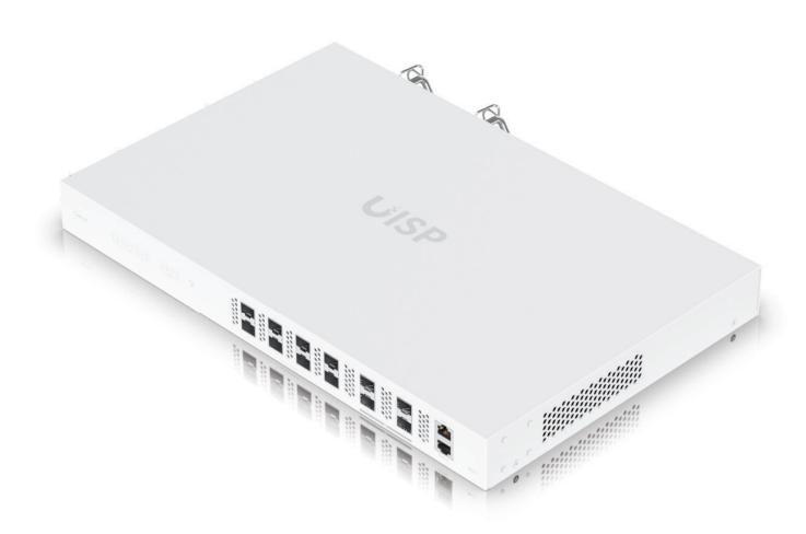
An eight-port optical line terminal, that can deliver 10 Gbps uplink/downlink speeds for over 2,000 subscribers.
